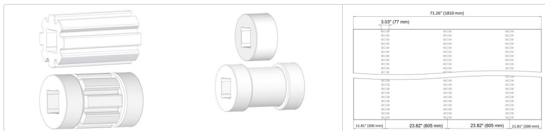
Sprockets Habasit® Cleandrive series
