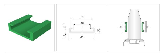
Standard materials: PE05 white High Density Polyethylene and PE10 black and green Ultra High Molecular Weight Polvethvlene.
