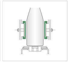
Standard materials: PE05 white High Density Polyethylene and PE10 black and green Ultra High Molecular Weight Polvethylene.
