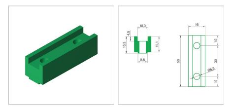
Standard materials: PE05 High Density Polyethylene (white color), PE10 Ultra High Molecular Weight Polyethilene (black and green color), PA6 Polyamide (white color), POM Polyoxymethylene (black color)
