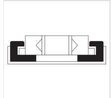
Standard materials: PE05 white High Density Polyethylene and PE10 black Ultra High Molecular Weight Polvethylene.
