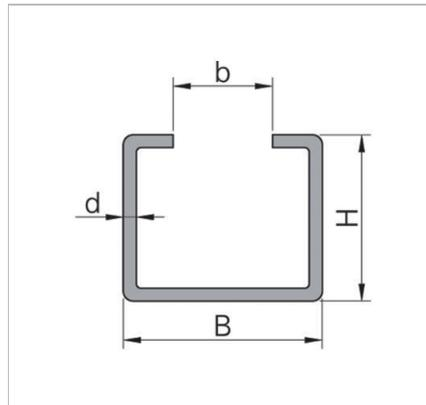
**Standard materials:** Galvanized steel and AISI 304 Stainless steel
