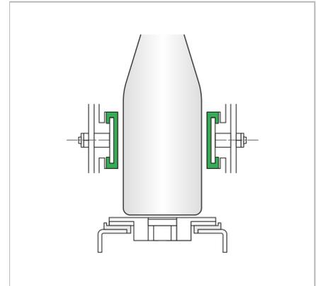
**Standard materials:** PE05 white High Density Polyethylene and PE10 black and green Ultra High Molecular Weight Polyethylene.
