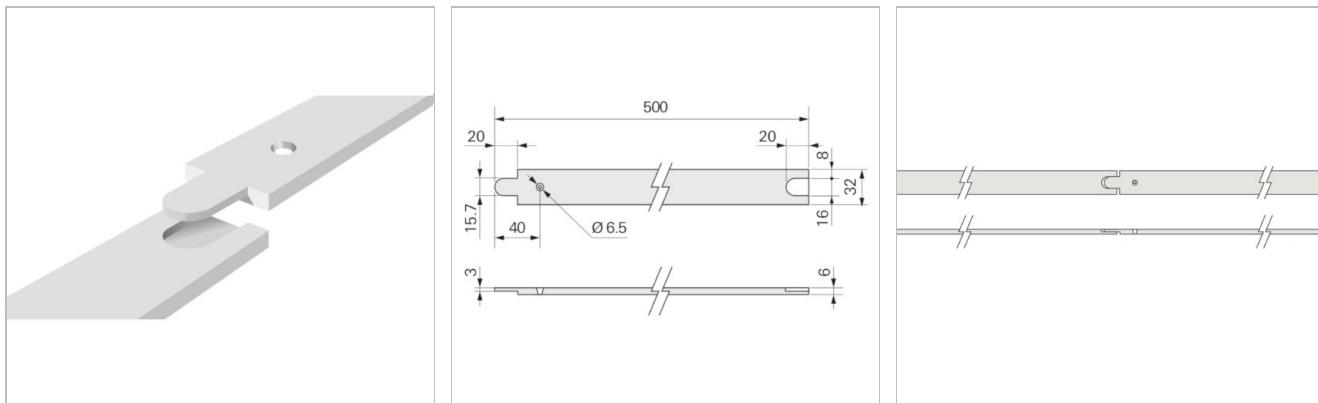
**Standard material:** PE03 High Density Polyethylene
