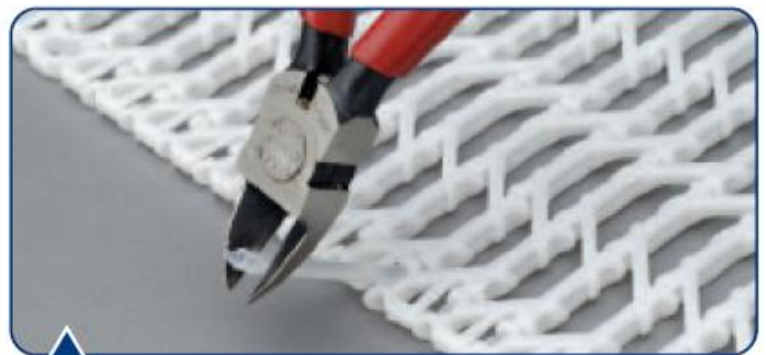
The rod will protrude on the opposite end. Pull on the exposed rod to draw the swedge head through the belt to disassemble.
