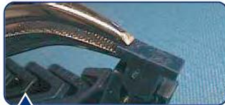
▲ Use nose pliers to put plug into position.
