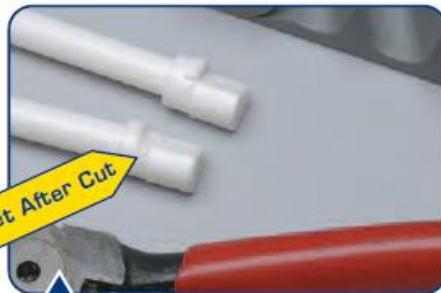
Be sure to cut "snap" off at the molded recess.
