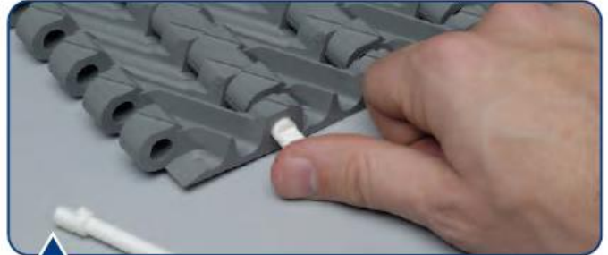
Insert rodlet — flat side up and tap into place with mallet (repeat process on other side of belt).
