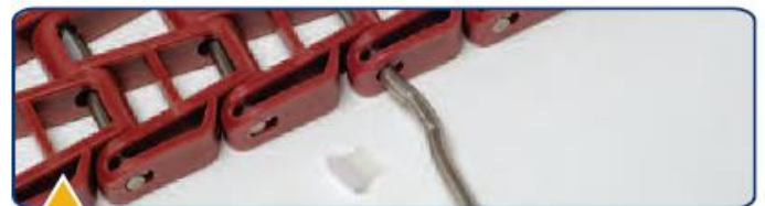
After the flag is removed, the rod can be pushed out with a punch or screwdriver.
