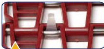
Insert the flag between the belt and the crimp in the rod with the thick part of the flag touching the belt.
