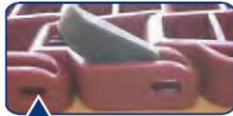
After rod is positioned, place plug and drive it in position with a hammer.
