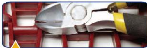
Use a pair of cutters to pull the flag into the belt until it is fully seated. Cut the excess flag off so that it is level with or below the top surface of the belt.
