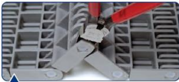
Insert clippers between the first and second finger of the belt on the headed side of the rod. [Bending the belt at the hinge will make it easier to insert the clippers, if bending is possible.]
