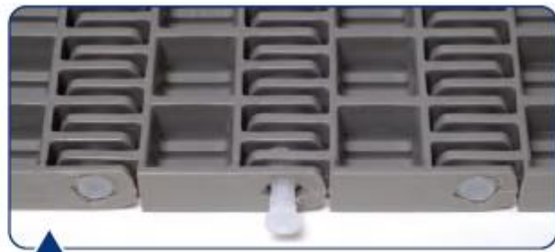
Pry out the head of the rod with the clippers. The rod can then be easily removed by hand.
