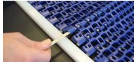
Insert rod, for easy rod installation, rod end must be beveled.
