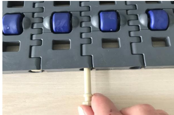
Insert rod. For easy installation rod end must be beveled.
