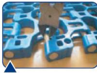
Use a gate cutter to grip the rod and force the rod to the outer side so that the outer finger is "deformed".
