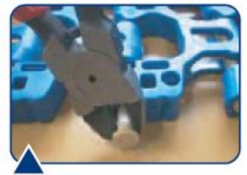
Use the gate cutter to pull out the rod completely.
