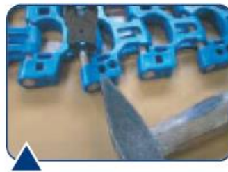
Use a hammer to hit the module (not the rod) so that the head of the rod is exposed.
