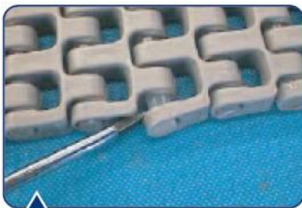
Use a small, flat blade screwdriver to bend open the belt and release.
