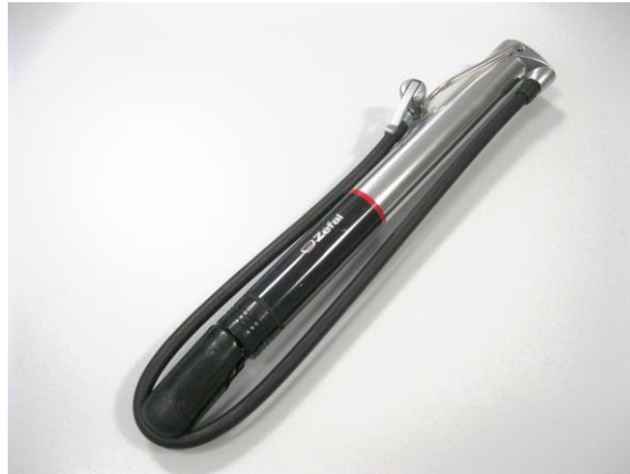
PRESSURE BAG INFLATION MANUAL PUMP. IT'S CONNECTED TO THE SCHRADER VALVE ON THE LOWER PRESS BEAM.
