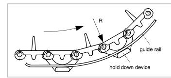
It is very important that the guide rail is very smooth, without joining. It is also important that enough clearance is provided to allow the belt to expand or shrink.
