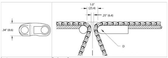
Inserts Note: Inserts may affect belt pull Nosebar or roller Diameter 0.75" (19.1 mm)
