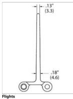
Standard flights are available in 1", 2", and 3" heights. Standard flight indent is 1" or greater from outside edge of belt
