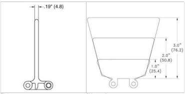
Flights Standard flights are available in 1", 2", and 3" heights. Standard flight indent is 1" or greater from outside edge of belt
