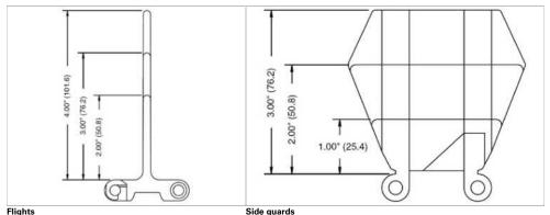
Standard flights are available in 2", 3" and 4" heights. Standard flight indent is 1" or greater from outside edge of
