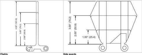
Flights Standard flights are available in 2", 3" and 4" heights. Standard flight indent is 1" or greater from outside edge of
