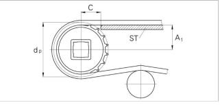
The distance **C** between the sprocket axis and the slider support **ST** is minimal 28 mm (1.1").
