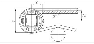
The distance **C** between the sprocket axis and the slider support **ST** is minimal 53 mm (2.1").
