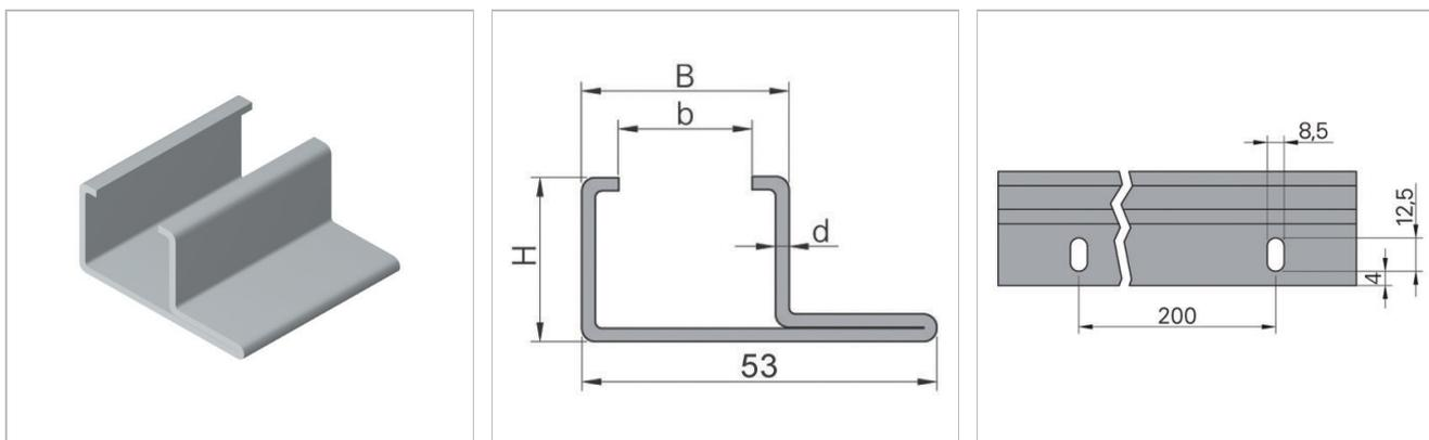
**Standard materials:** Galvanized steel, AISI 304 Stainless steel and Aluminum
