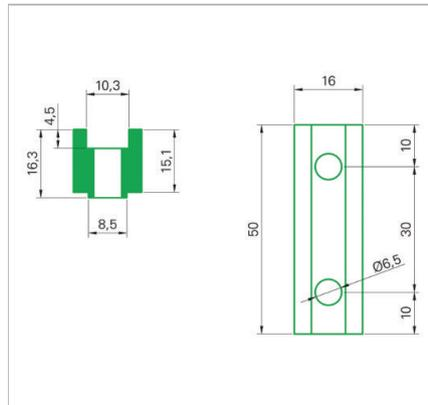
**Standard materials:** PE05 High Density Polyethylene (white color), PE10 Ultra High Molecular Weight Polyethylene (black and green color), PA6 Polyamide (white color) , POM Polyoxymethylene (black color)
