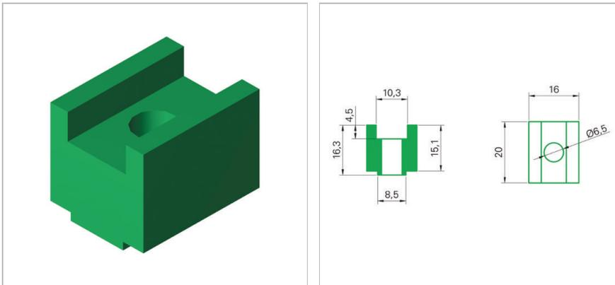
**Standard materials:** PE05 High Density Polyethylene (white color), PE10 Ultra High Molecular Weight Polyethylene (black and green color), PA6 Polyamide (white color) , POM Polyoxymethylene (black color)
