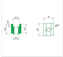
Standard materials: PE05 High Density Polyethylene (white color), PE10 Ultra High Molecular Weight Polyethilene (black and green color), PA6 Polyamide (white color), POM Polyoxymethylene (black color)
